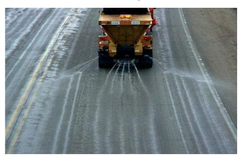
Blend GEOMELT® 55 with Na/Mg/Ca brines Apply at 20-30 gals / Ln mile(47-71 ltrs / kilometer)\*\* Reduced application rates 30% compared to Na Brine Reduce application rate for Frost protection - bridges Residual will last 4-6 days
